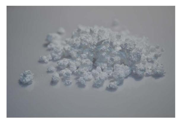
High Purity Alumina crystals (99.9855% Al<sub>2</sub>O<sub>3</sub>)
