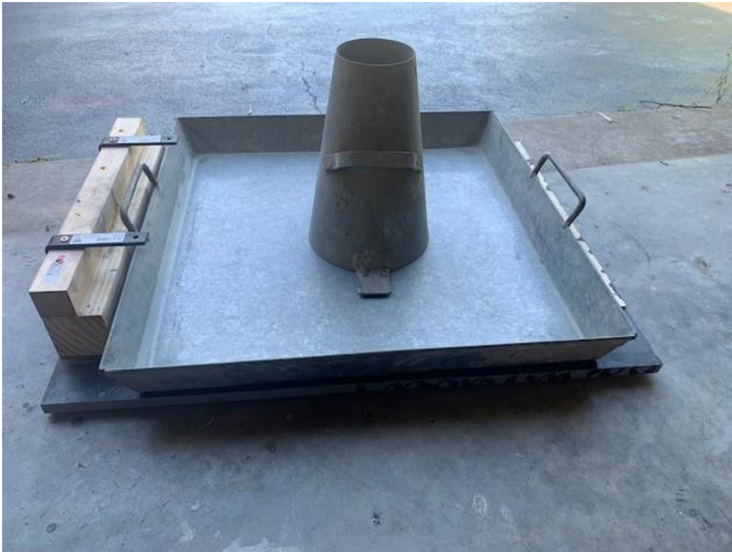
Figure 5.1c – Slump flow table with current available test equipment
