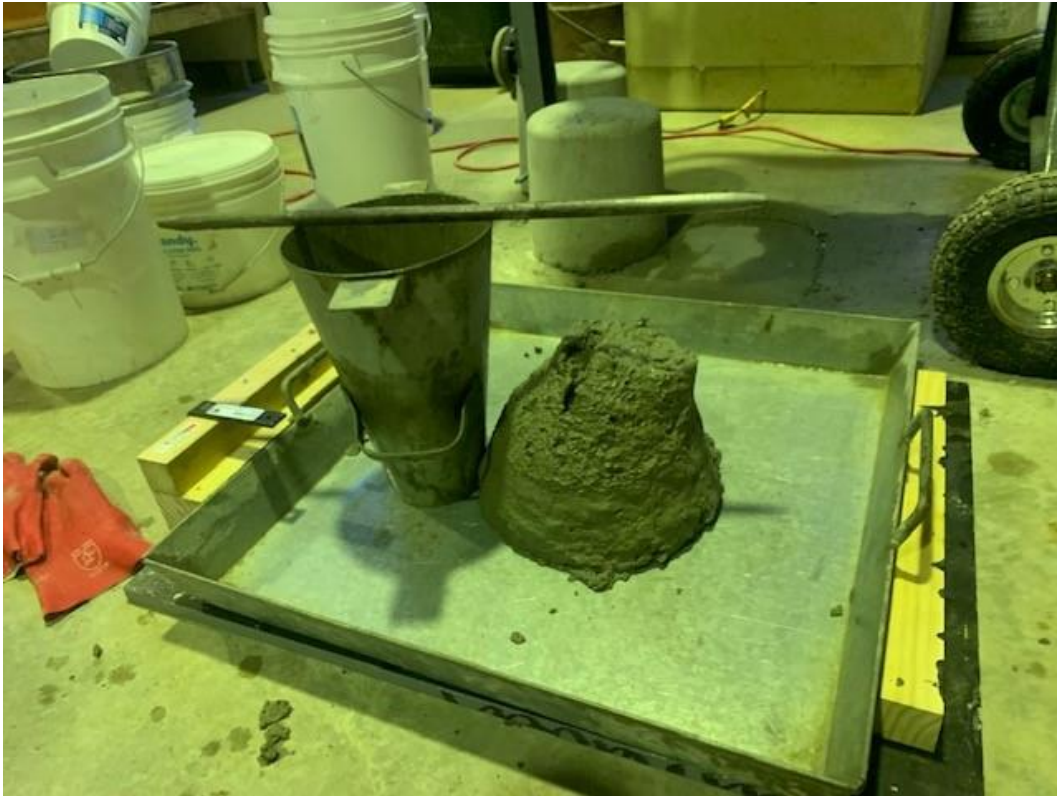
40Mpa Control – Slump
