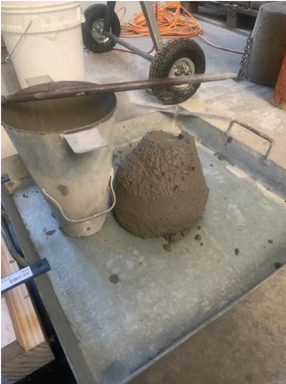
32Mpa Control Slump
