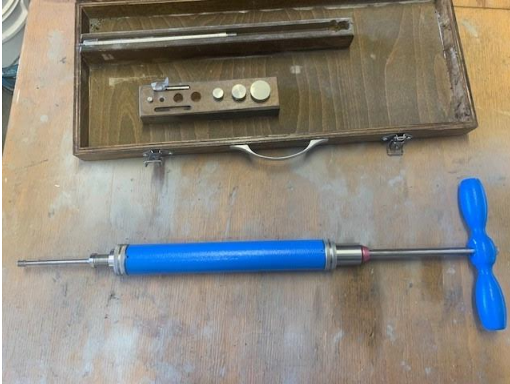
Figure 5.4a – Typical Penetration apparatus for initial and final setting time of mortars
