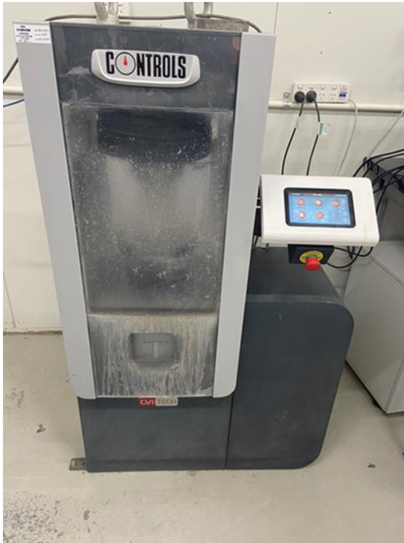
Figure 5.3a – Typical Compression machine used for compression testing of cylinders
