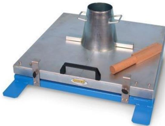
Figure 5.1a – Typical equipment used for testing to BS EN 12350-5
