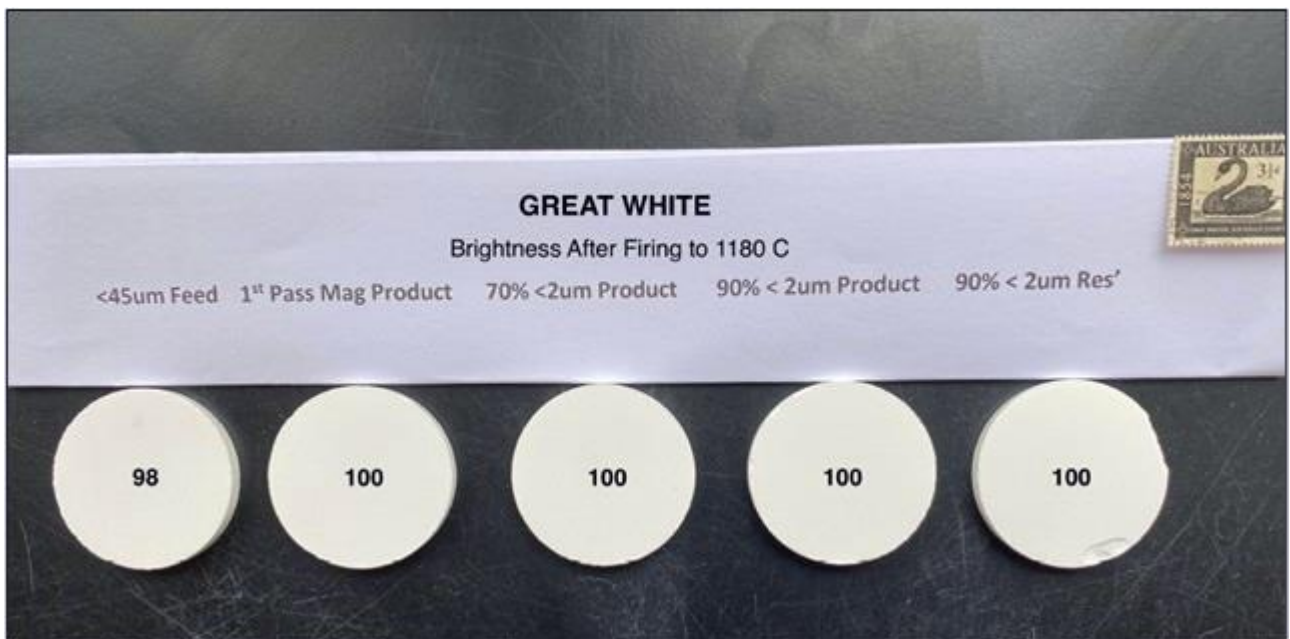
Figure 2 - Fired brightness discs from ceramic testing completed recently
